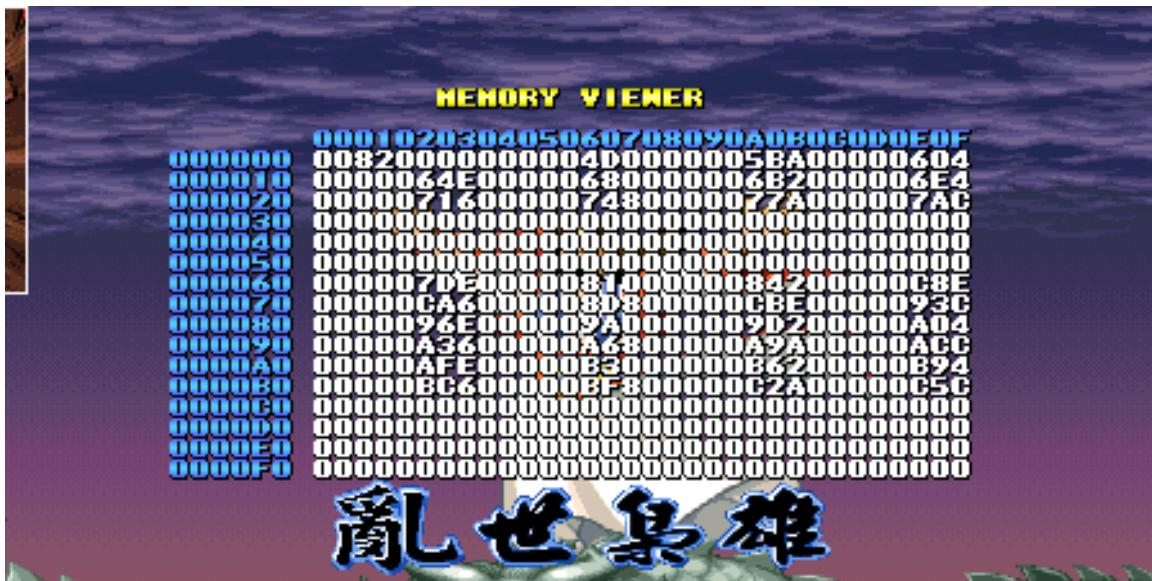
The memory viewer function is controlled by the P1 inputs. The display shows the current memory offset to the left (in blue) and across the top (00, 01, 02, ETC). The controls are as follows:
