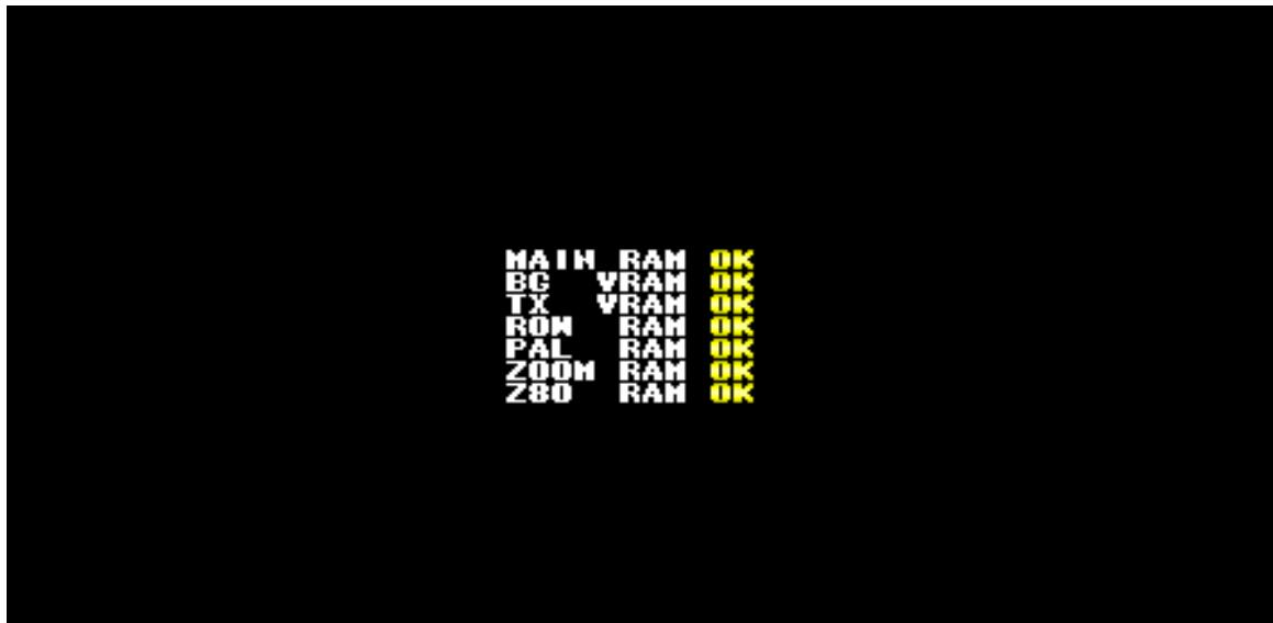
This screen tests all the main RAM regions of the PGM motherboard multiple times. Any failures are noted. This screen will display until P1 Button A is pressed. It can be triggered by enabling this option from the settings menu and rebooting the system. To loop this test, enable the ‘Test Mode’ dip (#0).
