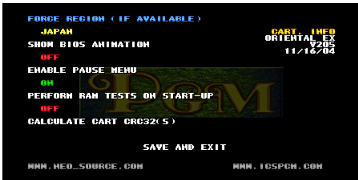
This menu can be accessed by setting the test (diagnostics) switch on start-up. Press up/down on the player 1 joystick to select the desired setting, and P1 button A to cycle through each option for that setting or by the in-game pause menu (section 3).
